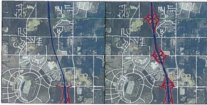
Figure 2. Example of Phase One results. Unedited highway intersection, left. Corrected intersection with access ramps, right.
